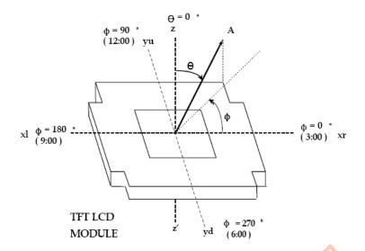
viewing angle is the angle at which the contrast ratio is greater than 10.the angles are determined for the horizontal or x axis and the vertical or y axis with respect to the z axis which is normal to the lcd surface.
